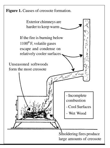
driest wood possible and using only small pieces of wood during mild weather when combustion is relatively slow. The stack temperature can be raised by insulating the stove pipe connection so that it cools as little as possible before reaching the chimney. Using an insulated pipe also aids in increasing the stack temperature.
