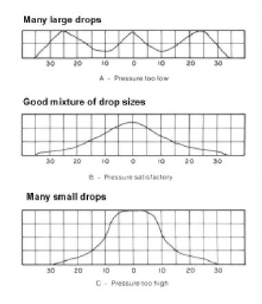
Figure 11. Variation in water application rate with horizontal distance (in feet) to the left and right of the sprinkler riser. The riser is located at distance "0".
