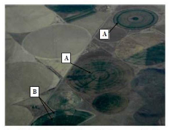
Figure 9. Poor center pivot uniformity due to malfunctioning pressure regulators (A) or incorrect nozzles on spans (B)
