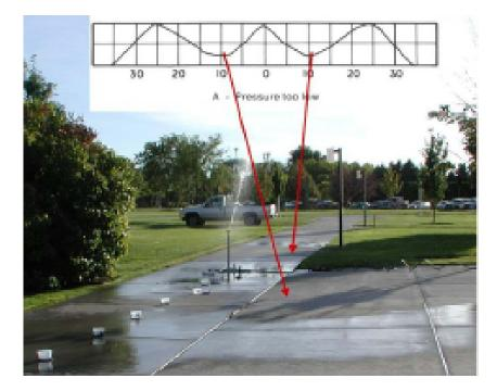
Figure 12. Water distribution from a sprinkler test using a brass nozzle at 20 psi system pressure for 20 minutes. Note the dry areas on the pavement corresponding to low areas in the theoretical distribution shown above.
