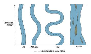
Figure 35. Descriptions of various stream sinuosity measurements. *Courtesy of Noah Kroese.*
