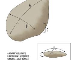
Figure 33. In a Wolman pebble count, you will measure the B-axis of the pebbles, which is the midlength axis. Courtesy of Noah Kroese..
