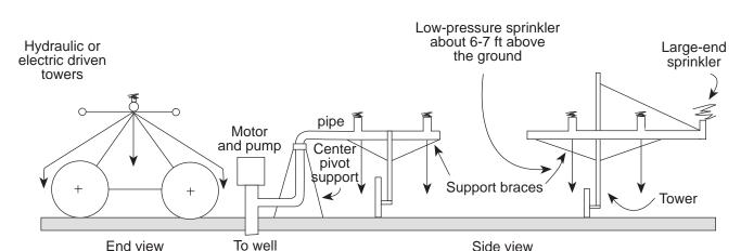
**Figure 2.** Mechanical-move sprinkler system: Self-propelled (center-pivot) lateral.
