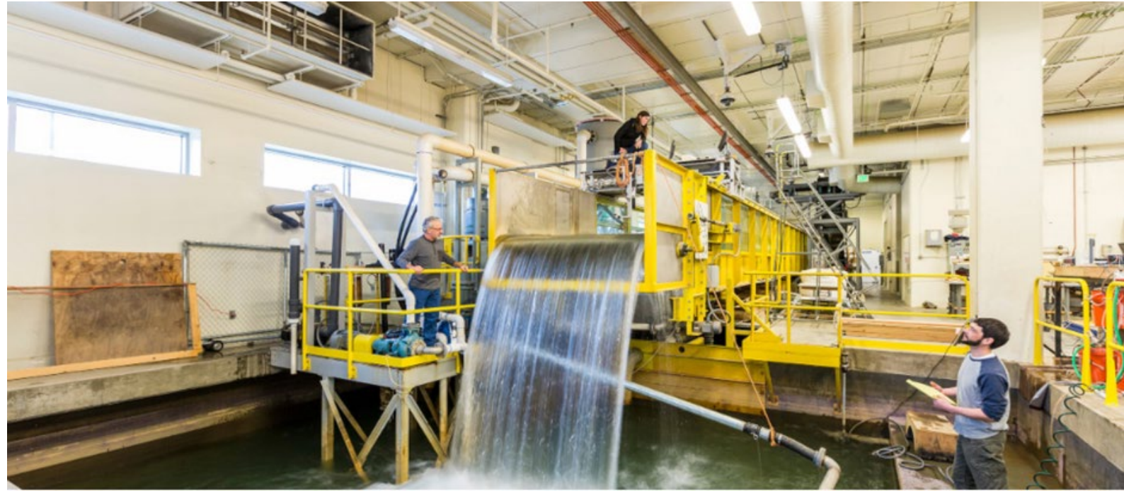
Sediment flumes in the center allow for advanced simulation of Idaho's streams and rivers.
