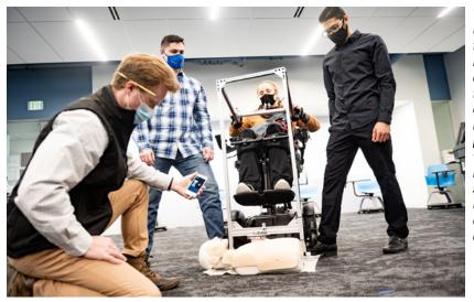
The team uses a training mannequin connected to a mobile app to record CPR performance, verify results and successful use of the custom device.
