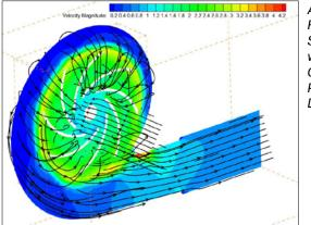
ANSYS Fluent Flow Simulation with Customized Pump Design
