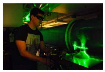
(Above) Mechanical engineering graduate student Rodrigo Padilla compiles lift and drag measurements using the new PIV system that allows users to visualize particles around a moving membrane (right).
