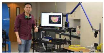
Paulo Yu uses the department's new 2D Particle Image Velocimetry system to study flow behavior of biofluids inside an aneurysm.
