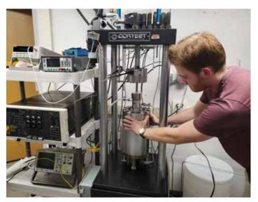
Graduate student Colin Burkhalter demonstrates the apparatus designed to performed fatigue and corrosion tests at high temperature and pressure using a high purification water circulation loop.
