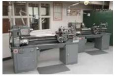
Acra precision engine lathes (left) were installed to replace 50-year-old manual lathes (above).
