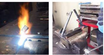
The triangle design consists of a 5-piece handle (left). Rebar was heated to bend the triangles into shape (above).
