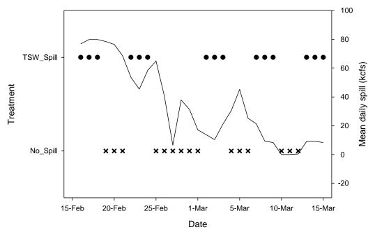
Figure 14. Spring spill test treatment blocks (symbols) and mean daily spill at McNary Dam from 15 February to 15 March 2015.
