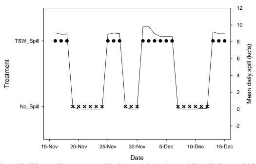
Figure 13. Winter spill test treatment blocks (symbols) and mean daily spill (lines) at McNary Dam from 15 November to 15 December 2014.
