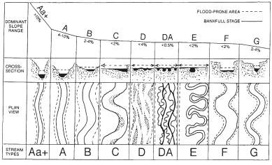
Figure 5. Rosgen stream classification identification diagram with the delineative criteria of stream gradient, channel cross-section, and sinuosity pattern (Rosgen 1996).
