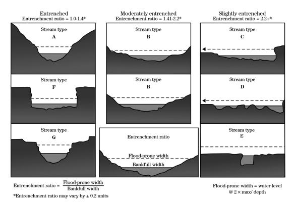
Figure 6. Examples of general channel shape, entrenchment diagrams, and entrenchment ratios for all Rosgen channel types (Rosgen 1996).
