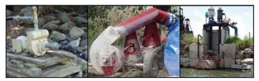
Figure 2. Examples of domestic, centrifugal, and turbine pumps.
