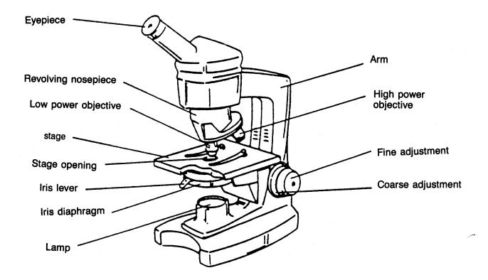
7. Underneath the stage is a *diaphragm*. The diaphragm regulates the amount of light entering the microscope. The diaphragm is adjustable for the type of lighting conditions used.
