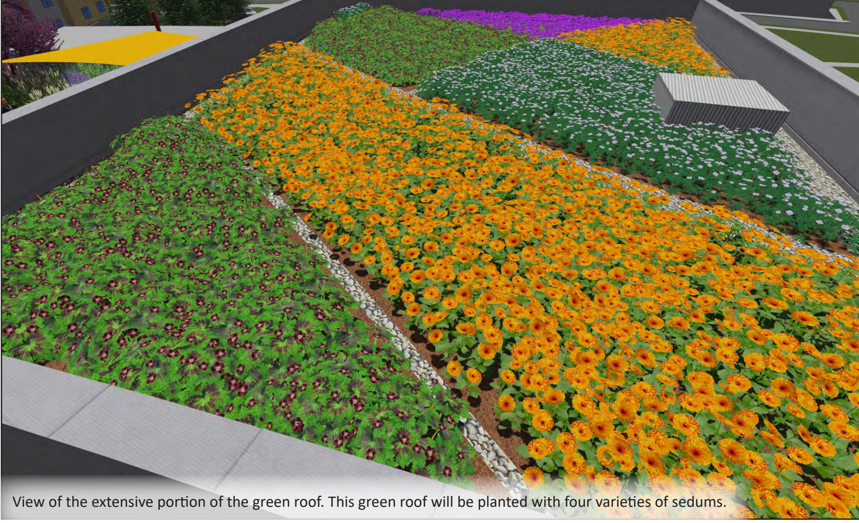
View of the extensive portion of the green roof. This green roof will be planted with four varieties of sedums.
